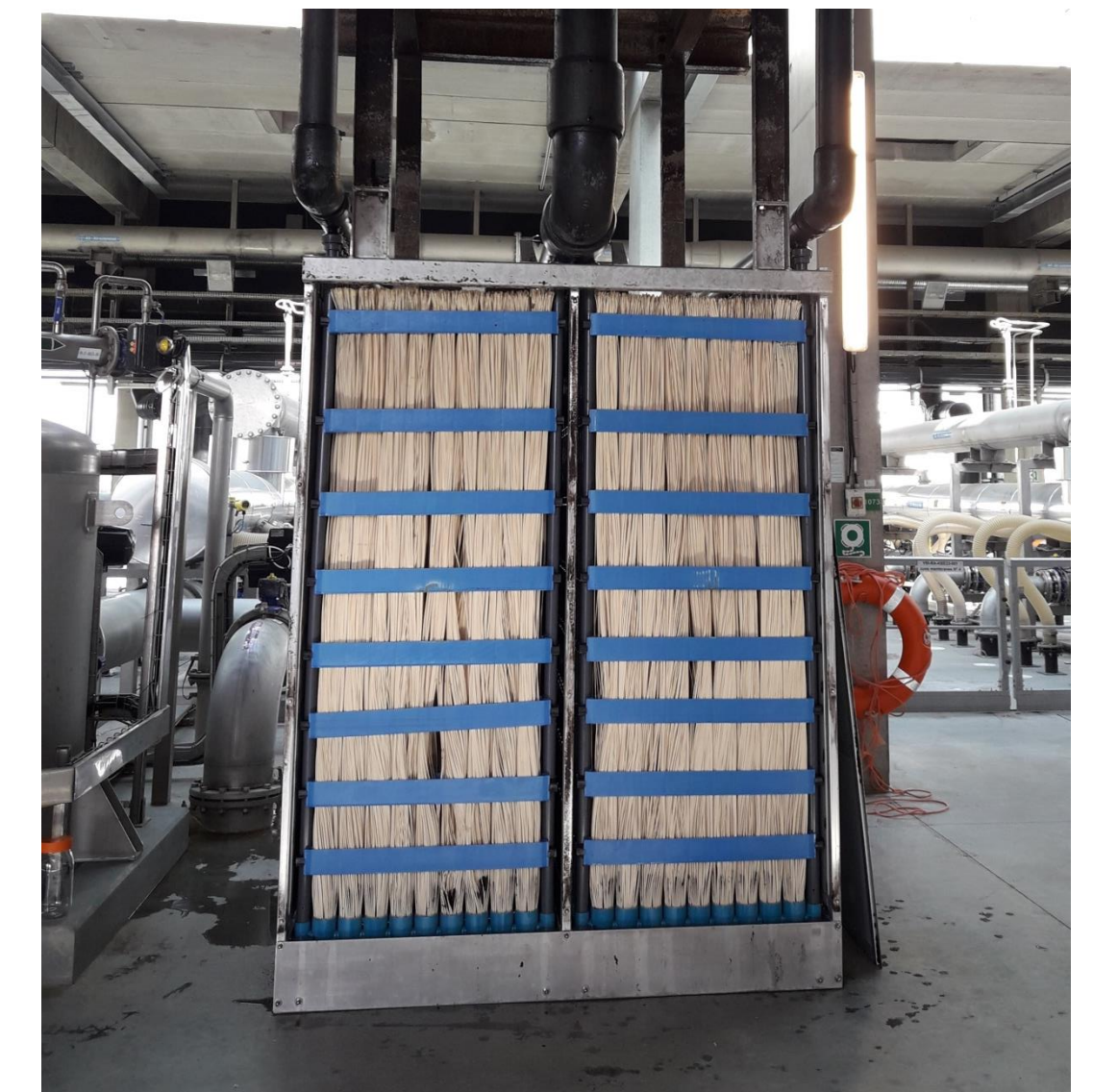
Fig 1. Extracted membrane module from full-scale MBR
